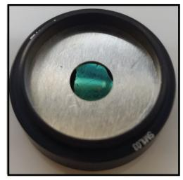
High-quality DAST has been the work-horse organic crystal for broadband, high-field THz genereation for several years. With a range of crystal thicknesses and extremely large aperture sizes available, we can meet your high-field THz generation needs. DAST is optimally phase-matched for pumping from 1.3-1.6 microns, but also provides good phase-matching from 1-2 microns.
